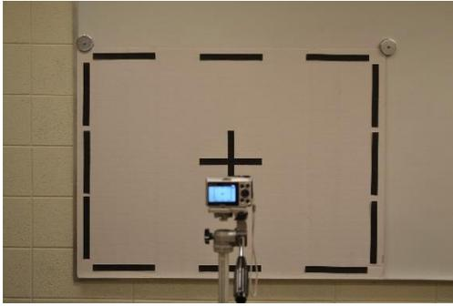
Figure 1. Target used to study variations in apparent length of segments located in different parts of the field of view.
