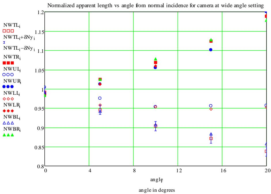
Figure 2. Apparent length as a function of angle from normal incidence to the target with the camera lens at its wide angle setting.
