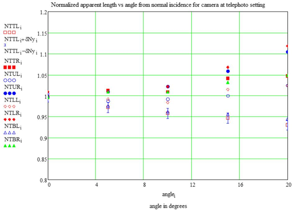
Figure 3. Apparent length as a function of angle from normal incidence to the target with the camera lens at its telephoto setting.
