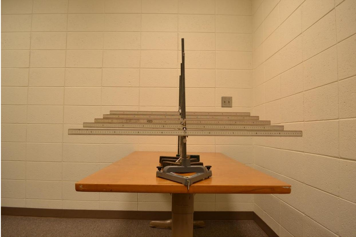
Figure 5. Meter stick array used to study parallax.
